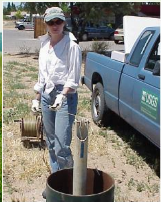
A USGS hydrologist collecting ground-water levels at the Sierra Vista monitoring well. Frequent and consistent measurements of ground-water levels are crucial for understanding the aquifer system and tracking water-level declines.
