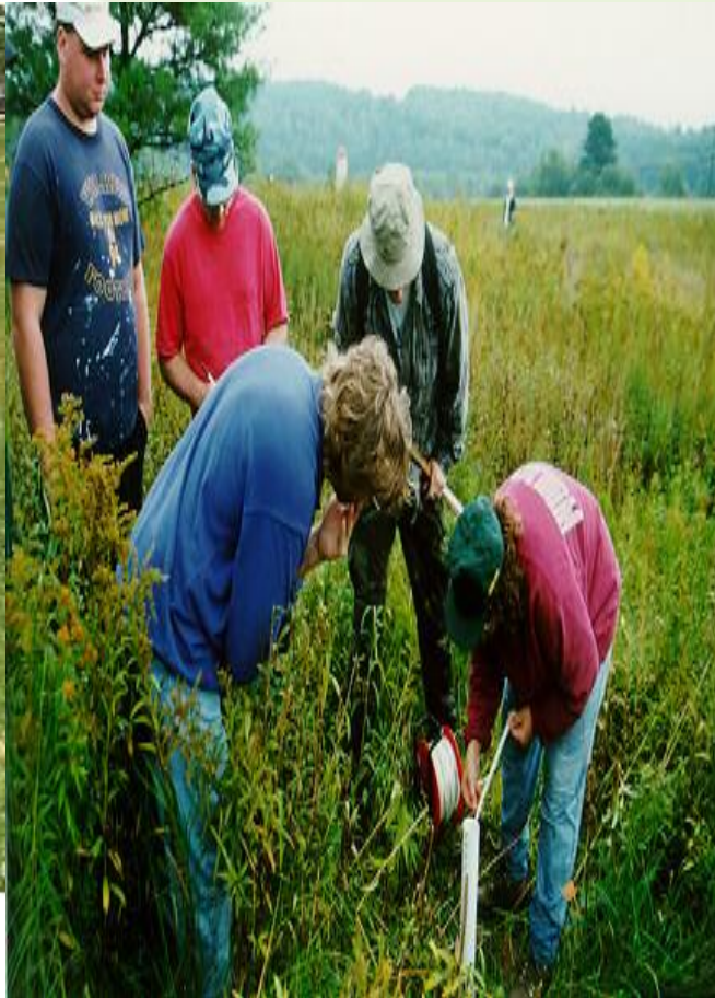
A USGS hydrologist collecting ground-water levels at the Sierra Vista monitoring well. Frequent and consistent measurements of ground-water levels are crucial for understanding the aquifer system and tracking water-level declines.
